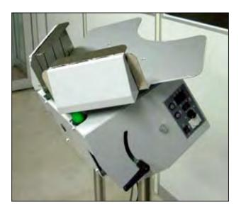
(3) When using the paper tray while setting it horizontally, load sheets of paper little by little (If the paper is loaded in mass, the tray receives the weight all at once, which makes it difficult to jog the paper properly).
