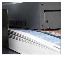
PATENTED FEEDING MECHANISM The patented "Tri-Suction Feeding Mechanism" reduces risks of double feeds and mis-feeds drastically, therefore it prevents paper jams and enhances productivity.
