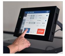
**INTUITIVE OPERATION** The 10" touch screen allows operators to set job programs and run the machine intuitively and instantly.
