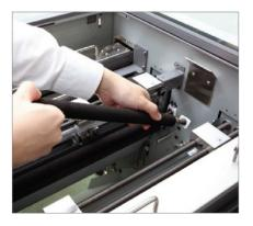
**EASY MAINTENANCE** The X Pro has detachable rollers, not only making cleaning easy, but it gives better access to components in case of a paper jam.
