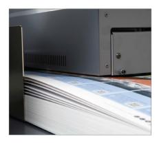
PATENTED FEEDING MECHANISM The patented Tri-suction Feeding Mechanism reduces risks of double feeds and mis-feeds drastically, which prevents paper jams and enhances productivity.
