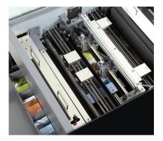
**ROBUST SLITTERS AND CUTTERS** The self-sharpening slitter and blade unit allows the machine to cut up to 400 gsm.
