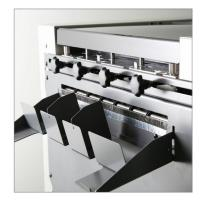
InstaSet BAR Unique InstaSet bar indicates and aligns slitter positions accurately and can be easily adjusted manually without tools.
