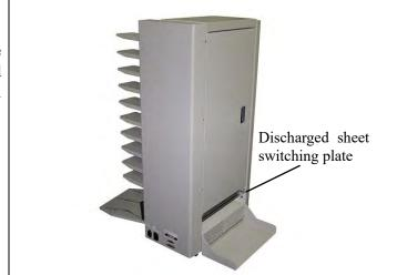
Switch the discharged sheet switching plate In Independent mode: The sheet collator is used alone.
