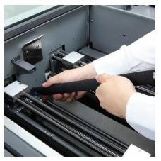
**EASY MAINTENANCE** The X and X Pro have detachable rollers, not only making cleaning easy, but gives better access to components.
