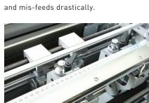
**JUMP PERFORATOR** Jump perforator allows you to perf the full length of the sheet or pre-determined measurements on the X Pro.
