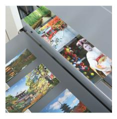
Flex mode allows operators to cut multiple size of cards from a page and add desired numbers of creases on these.
