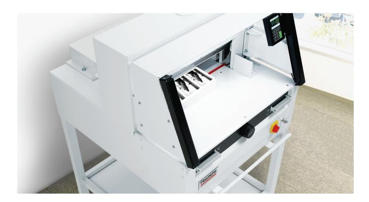
SCS (Safety Cutting System) is a combination of innovative design features which ensure the highest standards of safety. They protect the operator during the cutting process and while performing routine maintenance.
