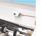
DOUBLE FEED DETECTION The double feed detection sensor prevents mis-feed papers (408A, 508A, 1800S).
