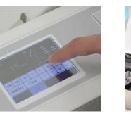
TOUCH-SCREEN The LED color touch-screen automatically sets up standard folds at the touch of a button (408A, 508A).
