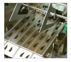
**DUAL PURPOSE INLINE & STANDALONE** Can be converted to run as a standalone machine allowing forms to be loaded from other printers into the large feed table.
