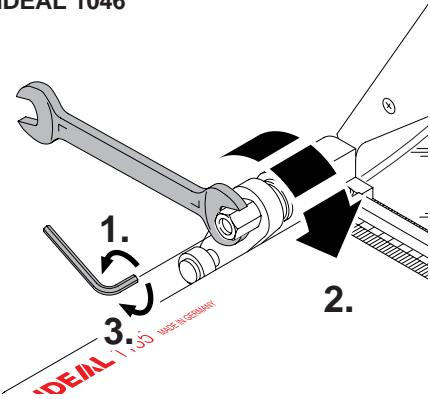
**GB** The machine has a **friction device** on the knife carrier. This insures, that the knife carrier cannot move down on its own. If it does re-adjust the friction device as follows:
