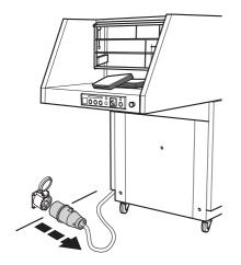
Remove the mains plug before cleaning the machine! Do not carry out your own repairs on the paper shredder! (See page 27).
