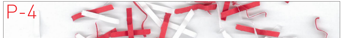
Material particle surface \leq .25 " squared and for regular particles: strip width \leq 1/4 " ( 3/16 " x 1 1/2 " particles, for example).
