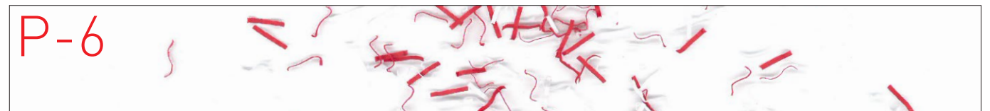
Material particle surface \leq .0156 " squared and for regular particles: strip width \leq 3/64 " ( 1/32 " x 1/2 " particles, for example).
