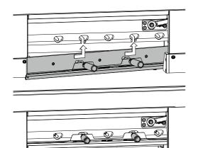
• Through the open slots, position blade with blade changing device at the top well over on the left and use the grips (5) for tightening.
