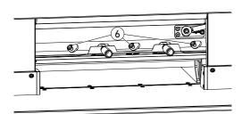
• Fit and tighten the 3 blade screws 6.
