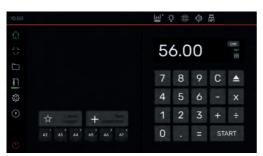
The unit of measurement can be changed by tapping in the dimension indicator on CM and also either in MM or inch.
