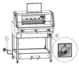
Plug in power cable (1) at the power socket. Ensure free access to mains.
