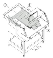
Paper installation at the back gauge ① and side stop to the left and right ②. Use the provided paper knock-up block ③ for adjusting paper stacks.
