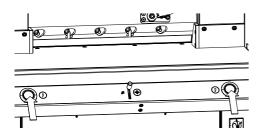
Simultaneously press both actuators, blade travels upwards at a reduced speed.
