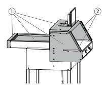
Dangerous machine parts are protected by guards and covered by panels (1). The machine may only be operated with all safety and panelling sections fitted and in particular
