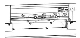
• Slightly slacken both grips (5) simultaneously and remove downwards blade and blade changing device. A Blade weight approx. 4 kg
