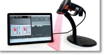
The VRCut solution consists of two independent modules that work together. The Impose module creates PDF documents formatted specifically to work with the VRCUT controller module. The controller module connects directly to the Triumph cutter moving the back gauge and visually guiding operators through the cutting sequence.
