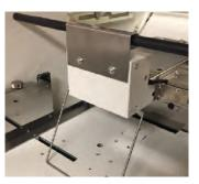
BELT FEED SYSTEM A belt fed, air suction system allows trouble-free feeding of coated stock (1800S).
