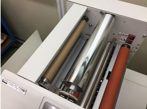
1. Set the foil you prepared on to the film shaft of the device. Firmly tighten the fixed color with a tool (supplied hexagonal wrench).
