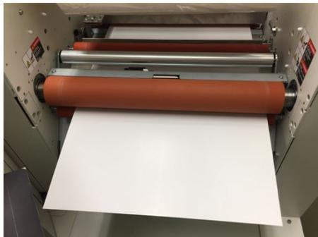
3. Insert the paper into the device as shown on the left figure. Open the pull roll lever at this point. Also, move the decurling bar back to its horizontal position.
