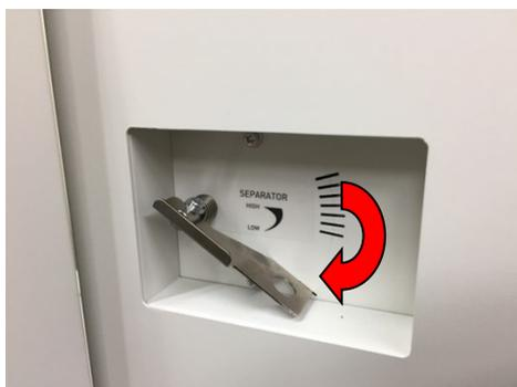
7. Close the feeder unit, lower the separating pressure adjustment lever to open, and insert the paper to the device by hand until it lightly hits the end.
