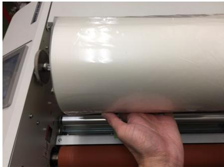
2. After setting the film on the film shaft, set the film to the film bearing of the device.
