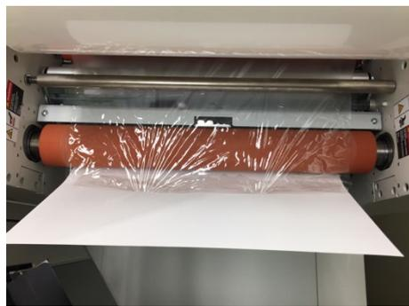
5. Confirm that the heat roller is well heated (212°F or more), and adhere the paper to the film as shown on the left figure. It is easy to adhere when the film turns transparent with heat.
