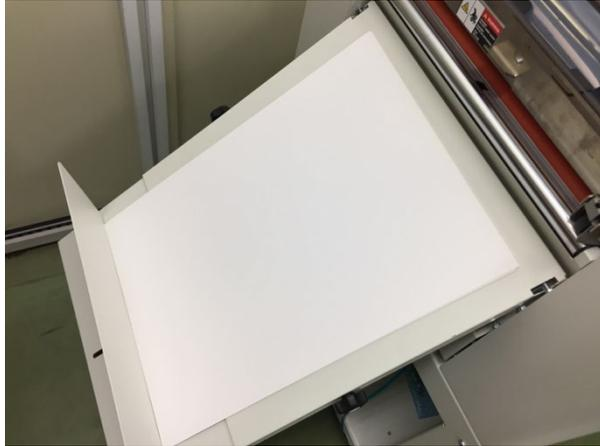
Firmly insert the tip of the stacker into the stacker attachment on the board at the machine side. Adjust the length of the stacker to the size of the paper to be processed. You can also adjust the installation height (two levels) and the angles (three levels each) to meet the corresponding capacity and size.
