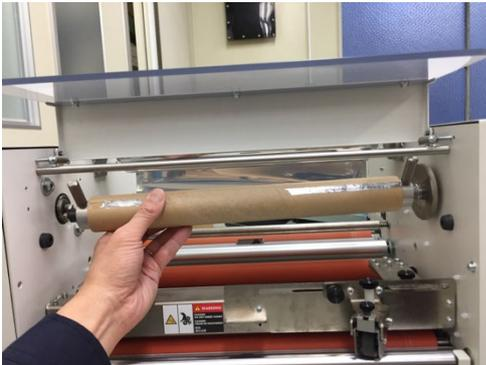
3. Set the paper tube for winding to the foil winding shaft as shown on the left figure. The setting is correct if it looks like the figure below at this point.
