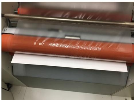
6. Using the manual feed switch to remove wrinkles from the film by transferring the paper. It will need about two sheets of ARCH B paper(12" x 18") to remove the wrinkles. Feed the paper to the position shown on the left figure using the manual feed switch. At this point, operate the manual switch, confirming whether the film and paper is firmly adhered or if the film is extending beyond the paper.
