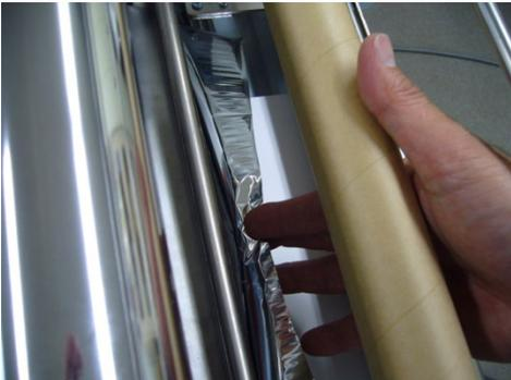
7. Press the paper and foil so that the inserted paper and foil would come out from the back side of the pull roller. If you can catch the foil as shown on the left figure, pull out the edge of the foil. Then, remove the paper as it will not be necessary.
