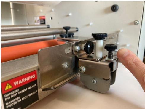
12. Adjust the decurling bar to the optimal position depending on the thickness of the paper.
