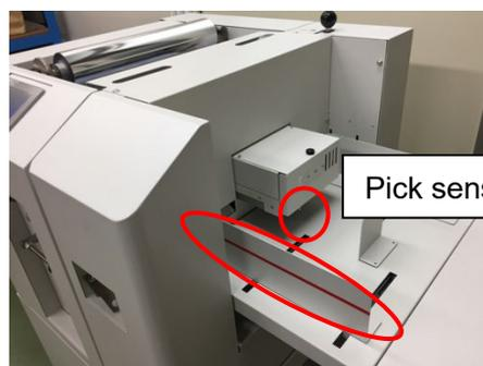
Set the papers and adjust the feeder tray paper guide to the width of the papers. Make sure the papers are inserted until it stops and that the rear end of the papers is aligned. Then, after confirming the papers are correctly installed, set the paper fixing guide to the rear end of the papers.
