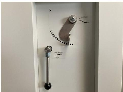
13. Finally, finish setting the film by lowering the pull roll lever.
