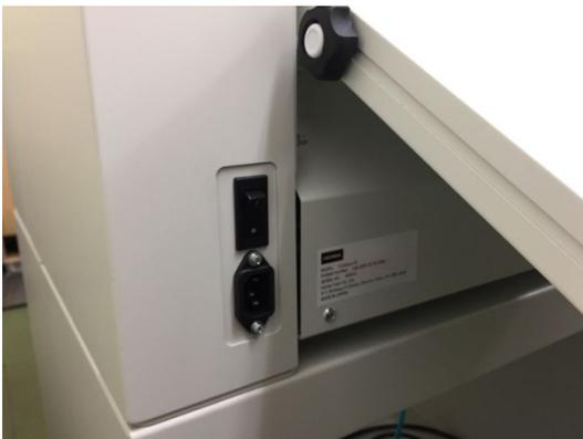
Firmly insert the power cable into the power socket at the bottom rear side of the main unit.
