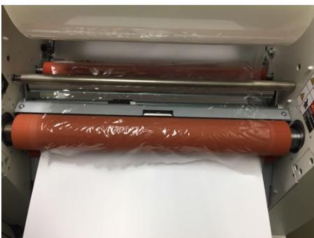
4. Pull out the film end for about 12inch, and set it on the heat roller as shown on the left figure.
