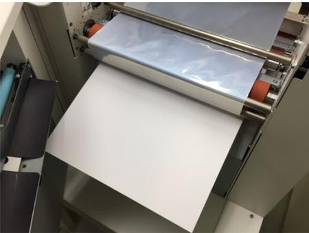
6. Insert a slightly thick paper into the device, pressing the foil as shown on the left figure. Set the pull roll lever upward at this point.
