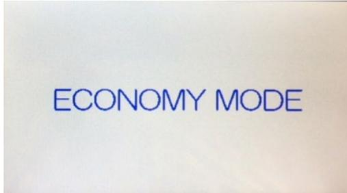
The machine will switch to the eco-mode if laminating/glazing is not processed or no button is pressed on the operation panel for more than 30 minutes.
