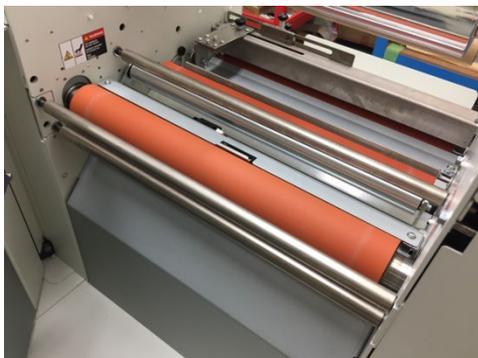
4. Set the guide dedicated for the foil as shown on the left figure. The setting is correct if it is set like the picture below.
