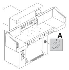
Paper cutting test. If the last sheet or several sheets are not completely cut, gradually turn the knob for blade depth adjustment (**A**) 1/6 turn to the left until the paper is cut along the entire length. Do not set too low as blade will soon become blunt.
