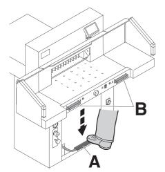
The clamp moves automatically when cutting is activated. The paper can be pressed in advance, with the foot pedal (**A**). Cutting is activated by pressing both buttons (**B**) on the front table.
