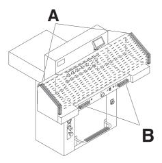
The cutting action, which is dangerous to the operator, is protected by a two-handed control system (**B**) and safety beam guard (**A**).
