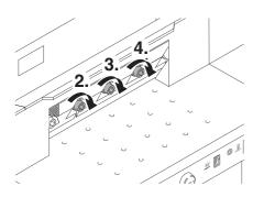
Tighten the remaining 3 blade screws beginning from the left.
