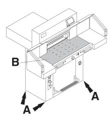
The machine is mobile on castors. Align the machine as followes:
