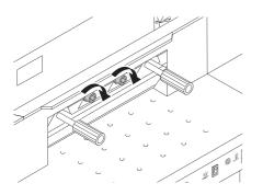
Tighten the middle blade screws.
