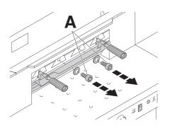
Remove the remaining two blade screws (A).
