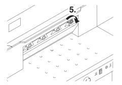
Tighten the blade screw which is visible at the right.
