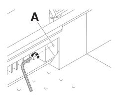
Does not cut through the last sheet.  $\rightarrow$  Reset the cutting depth (A) ...
