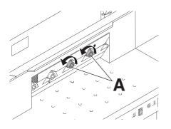
Loosen slightly the blade screws (**A**) so that the blade slides onto the cutting stick.
