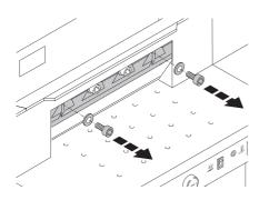
Remove both outer blade screws.
