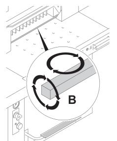
... or turn / replace the cutting stick (**B**). (See page 29 "Blade and cutting stick replacement").
