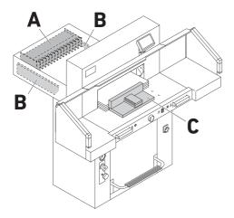
The stack of paper can be placed against the back gauge (**A**) and the left or right side stop (**B**). Use the supplied paper knock-up block (**C**) to move the stack of paper.
