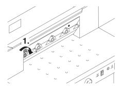
Tighten the left-hand blade screw while applying downward pressure.
