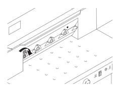
Screw in slightly the left blade screw.
