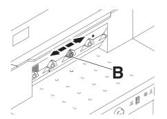
Push the blade with the blade screw (**B**) as far as possible to the left or right and then centralize them.  $\rightarrow$  The blade must rest on the cutting stick.
