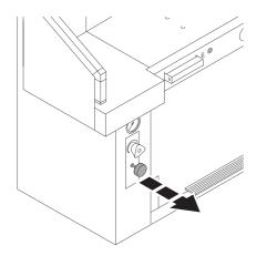
Pull out blade locking key  $\rightarrow$  blade moves to the top.
