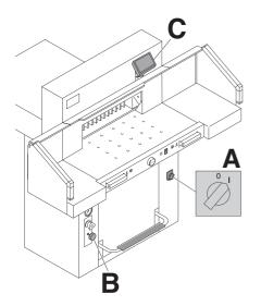
Display (**C**) is pivotable. By loosing the allen head screw (**D**), (allen wrench is in the tool box) the display can be pivoted within the elongated hole. Tighten allen screw again. Position the main switch to "I" (A). Blade locking facility (B) must be pulled out. Press  $\frac{1}{2}$  (C).  $\rightarrow$  Machine will automatically go to the start position. The machine is now ready for use.
