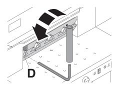
Remove the left blade screw ( $\boldsymbol{\mathsf{D}}),$  using the extension.
