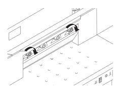
Slightly screw in outer blade screws.
