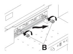
Simultaneously slightly loosen both handles (**B**) and remove blade with blade changing tool. **Weight of blade approx. 5 kg.**
